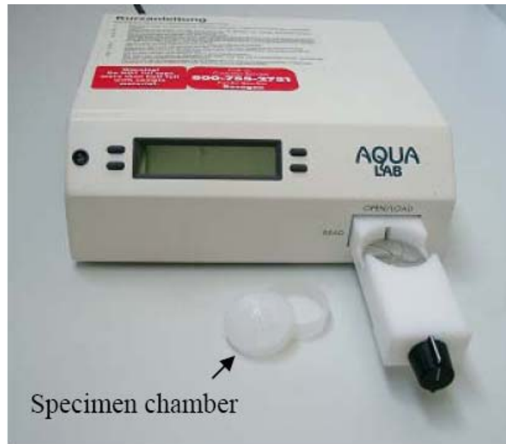
Figure 4.12 The chilled-mirror hygrometer (AQUA LAB) used in this study.
