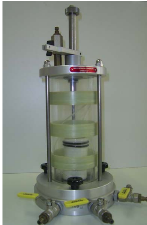
Figure 4.10 Triaxial cell setup used in isotropic consolidation test.
