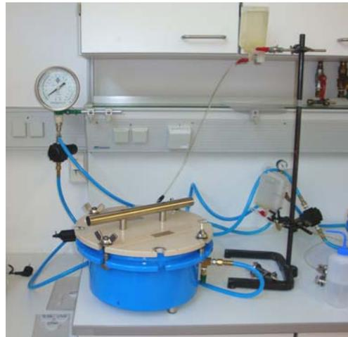
Figure (4.39) Photograph of the pressure plate
