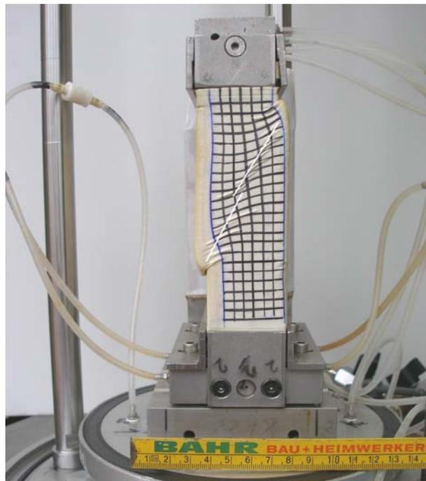
Figure (5.10) Shear band with two inclinations on the  $\sigma_2$  plane
