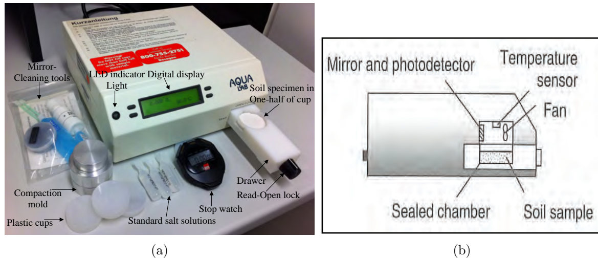
Figure A.1.: Chilled-mirror hygrometer device: (a) Device set up and (b) Schematic plot.
