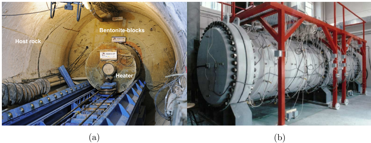
Figure 2.17: (a) Full-scale Engineered-barrier Experimental (FEBEx) performed at the Grimsel Test Site (GTS, Switzerland) (Villar et al., 2005) and (b) full-scale mock-up test in laboratory (Martin & Barcala, 2005).
