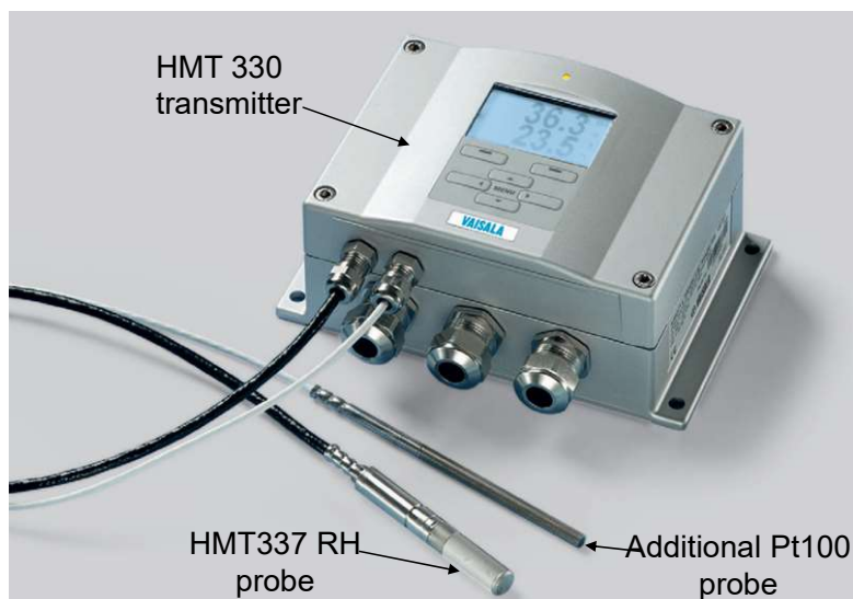
Figure 4.11: VAISALA HMT337 relative humidity sensors with additional Pt100 sensors
