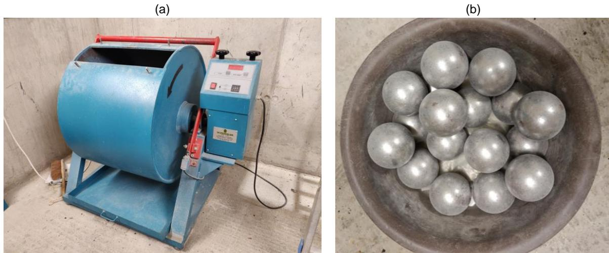
Figure 4.3: (a) The Los Angeles abrasion device adopted for crushing glass beads, (b) steel charges for crushing
