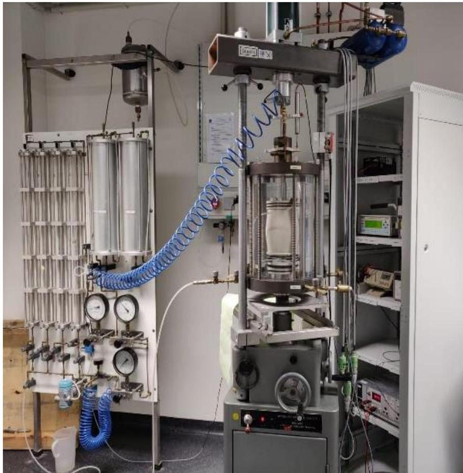
Figure 4.5: Triaxial device used for the various monotonic triaxial experiments
