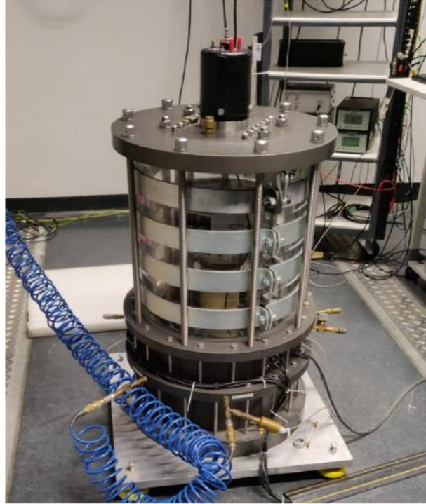
Figure 4.9: The Resonant Column device at Ruhr-Universität Bochum
