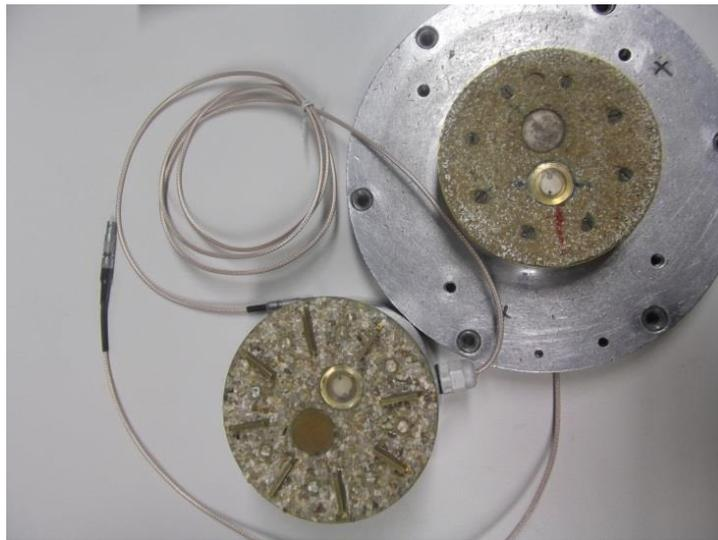
Figure 4.12: The top and bottom caps of the specimen with a piezoelectric compression element installed
